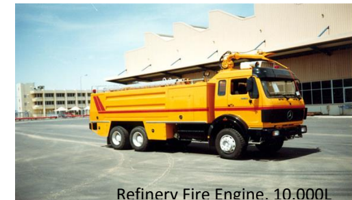
Refinery Fire Engine, 10.000L
